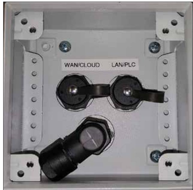
Figure 2 – AC Power and Data Connections in side box
