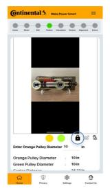
**Pulley center distance:** Measure the diameter of the pulley, the center distance and the wrapping angle from a picture. Keep the camera of your mobile device straight to the picture in a vertical, straight up position and watch for the app to reach 90 degrees, and then take the picture of the pulley system. You may capture your screen once the position and diameter of the pulley are set.
