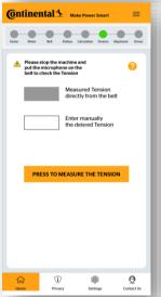
**Tension2Go:** Measure the tension value of your drive system in a very fast, easy and intuitive way. Enter the desired tension manually and press the measured tension button, while holding the phone ½ inch above the belt span, and "pluck" the belt. The real tension will be measured within 15 seconds. View results and make tension adjustments as needed.
