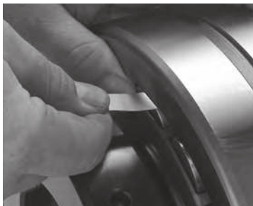
Fig. D-7. Measure RIC before installation.
