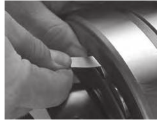
Fig. D-3. Measure RIC before installation.
