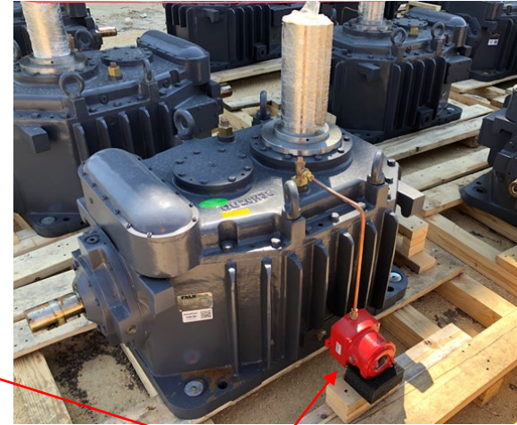
Factory-mounted oil level switch
