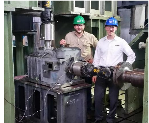
Pictured: Falk 2310CTA under test Rexnord Gear Product Manager Rexnord Manager of Test Services
